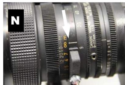
9. Engage the gears by sliding the focus motor into the lens gear then tighten the black knob to secure it. If the gears don't mesh perfectly, rotate the focus ring on the camera slightly so the gears mesh. **See Fig O**
