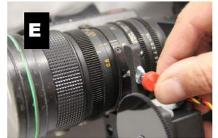
3. Use the wing nut to squeeze the bracket against the lens for a tight secure fit. See **Fig F**
