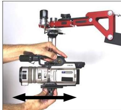
5. **HORIZONTAL BALANCE:** Balance the camera horizontally by sliding the camera forward or backward as shown above. Loosen the mounting knob slightly to allow the camera to slide.
