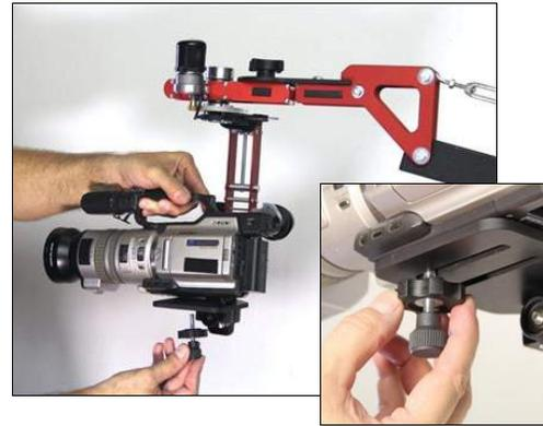
3. Use the camera mounting hardware provided to attach the camera to the camera cradle of the head. Drive the long screw deep into the camera, then use the lobe knob to jam it firmly in place
