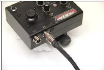
13. Use the Extension Cable to connect the Y cable to the Joystick controller. Plug the male end into the Y cable and the female end into the Joystick.
