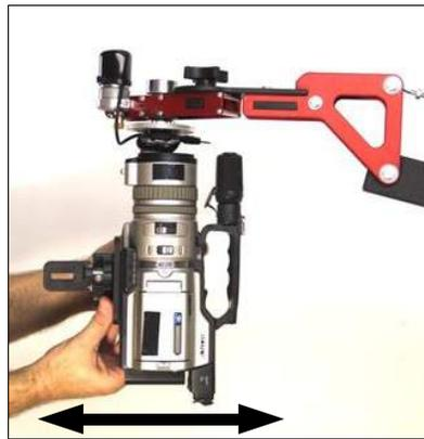
9A: You may find it easier to point the camera straight upward and slide the camera cradle left and right. From this position, moving the cradle left to right is actually balancing between the top and bottom of the camera.
