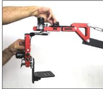
2. Use the knob to attach the head to the camera platform of the Skinny Jib. You have the option to mount the head in over or under slung position.
