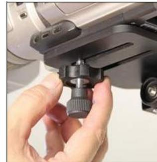
6. After achieving good horizontal balance, re-tighten the camera firmly to the platform.
