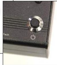
14. Connect the power supply to the Joystick and use the power button to turn the unit on and off.
