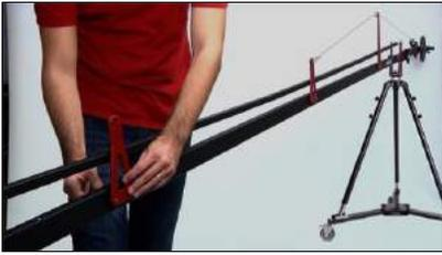
19. To achieve the 12' configuration add another lower Extension Beam and upper Para Extension Beam to 8' configuration.
