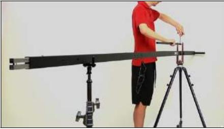
10. Add one Extension Para Beam for each Extension Beam added. One for the 8' configuration and a second one if you are building the 12' configuration.
