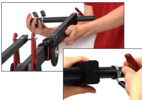
26. Attach the counter weight bar to the Tail End of the Jib. Use the hex tool to tighten the set screw (at butt end) to secure it in place.
