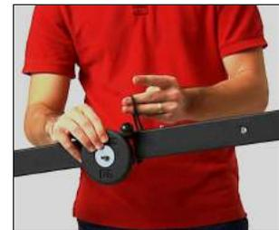
25. Attach the sliding counter weight to the Tail beam of the Jib via the bungee straps
