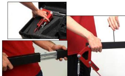
8. Use the Camera End Beam from the hard case and slide it over the expansion joint.
