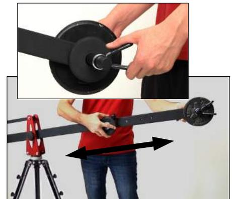
28. Add or subtract weights to achieve camera balance. Use the spring clips to secure them and the adjust the Sliding Coun-
