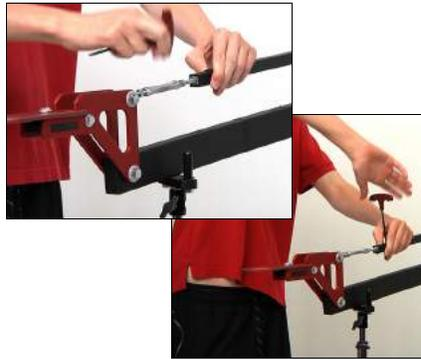
11. Connect the Turbuckle end on the Camera Platform beam to the female end of the upper Para Beam. Use the Hex tool to drive the set screw down to secure the connection.
