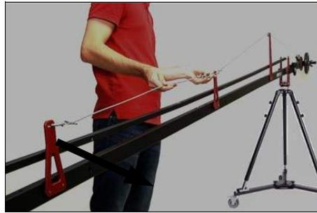
20. Add the short cable between the two Extension Beam Cable Hitches
