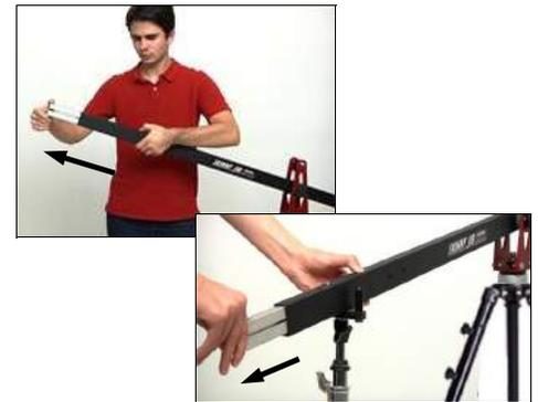
6. Pull out the expansion joint from the end of the Center Jib Beam until the spring pin clicks into place.
