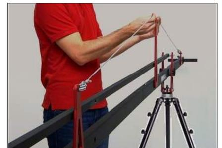
18. Lift the slack in the cable over the roller of the Cable Pole.
