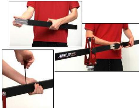
5. Pull the expansion joint from the 2' Tail Beam until the spring pin clicks into place.. Insert it into the female end of the Center Jib Beam. Use the hex tool to expand the joint and secure the connection.
