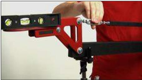
23. Place the provided level on to the camera platform. Use the turnbuckle to adjust the platform and achieve level.
