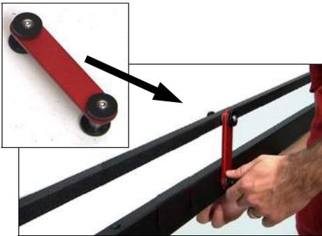
13. Use the Swing Arm to support the sag of the Para Beam. Remove the knobs and place the larger spacer in the lower Extension beam and place the smaller spacer in the upper para beam. Secure it by re-attaching the knobs.
