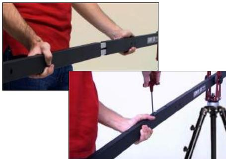
7. Add 1 Extension Beam for the 8' configuration. Use the Hex tool to tighten the connection firmly.
