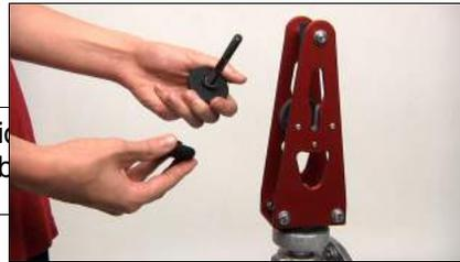
2. Remove the Center Pivot bolt from the center post by unscrewing the soft grip knob on the end.
