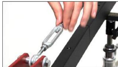
24. Finger tighten the nuts against the turnbuckle body to secure the setting. Wrench tighten for more rigidity.
