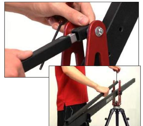
9. Connect the male end of the 4 Para Beam to the center post. Use the Hex tool to screw the para beam set screw and secure it into place.
