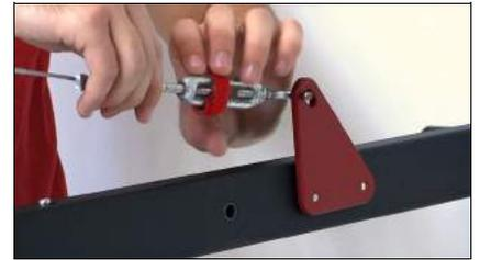
22. Use the turnbuckles to tighten or loosen the slack in the suspension cables.
