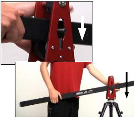
4. Run the Center Pivot Bolt through the Beam to the other side of the Center Post. Use the wide space for easy bolt alignment.
