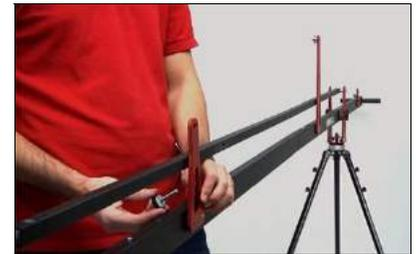
15. Attach one of the two Extension Beam Cable Hitches to the first Extension Beam.
