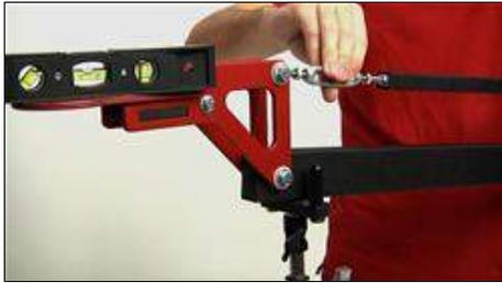
11. Place the provided level on to the camera platform. Use the turnbuckle to adjust the platform and achieve level.
