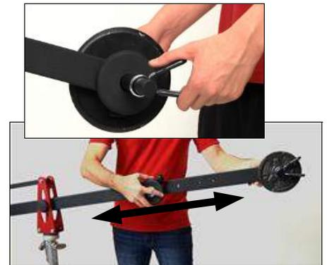
16. Add or remove weights to achieve camera balance. Use the spring clips to secure them and the adjust the Sliding weight for micro adjustments.
