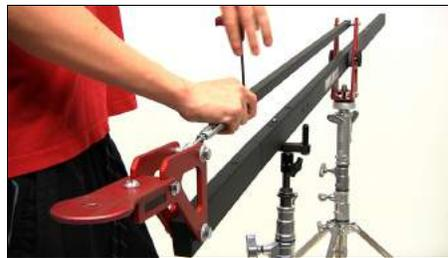
10. Connect the Turnbuckle on the Camera Platform beam to the female end of the Para Beam using the Hex tool and set screw.
