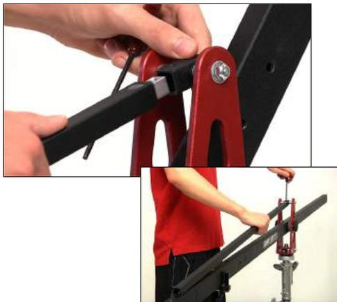
9. Connect the male end of the 4 Para Beam to the center post. Use the Hex tool to screw the para beam set screw and secure it into place.
