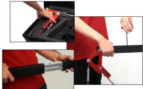
8. Use the Camera End Beam from the hard case and slide it over the expansion joint.
