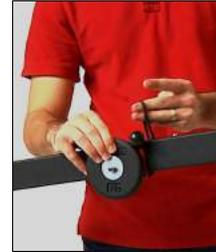
13. Attach the sliding counter weight to the Tail beam of the Jib via the bungee straps
