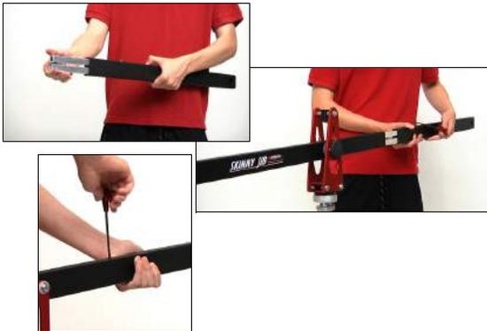
6. Pull the expansion joint from the 2' Tail Beam until the spring pin clicks into place.. Insert it into the female end of the Center Jib Beam. Use the hex tool to expand the joint and secure the connection.
