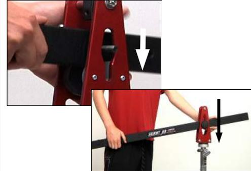
5. Run the Center Pivot Bolt through the Beam to the other side of the Center Post. Use the wide space for easy bolt alignment.
