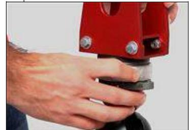
2b. For 100 or 75 mm Bowl Mount Tripods. Use the adapter plate and hardware (included).
