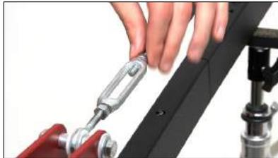
12. Finger tighten or use the provided wrench to tighten the nuts against the turnbuckle body to secure the setting.
