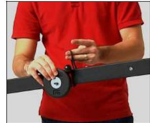
13. Attach the sliding counter weight to the Tail beam of the Jib via the bungee straps
