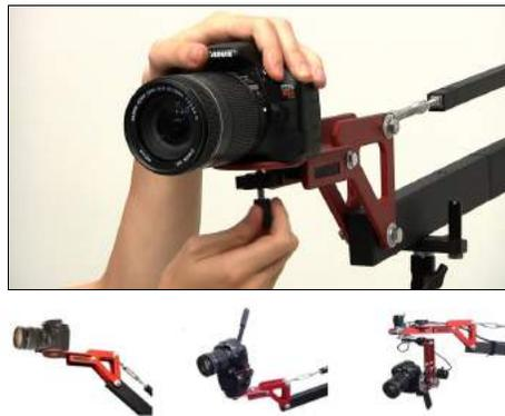
15. Attach camera. You can attach directly or via a fluid or motorized pan tilt head.
