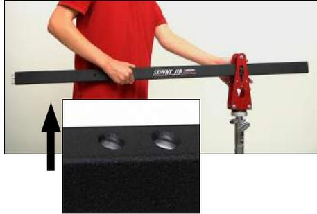
4. Place the 4' Tail Beam (w logo) thru the hallow middle of the center post. Position it so that the holes on the beam's edge are facing upward.
