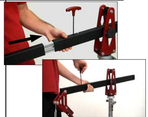
8. Slide the Camera End Beam over the expansion joint. Use the T Handles Hex tool to expand the expansion joint and create a firm connection.
