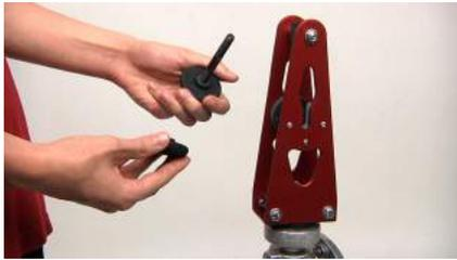
3. Remove the Center Pivot bolt from the center post by unscrewing the soft grip knob on the end.
