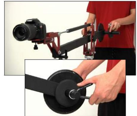
16. Add or remove weights to achieve camera balance. Use the spring clips to secure them and the adjust the Sliding weight for micro adjustments.
