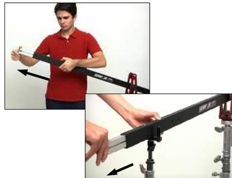
7. Pull out the expansion joint from the end of the Center Jib Beam until the spring pin clicks into place.
