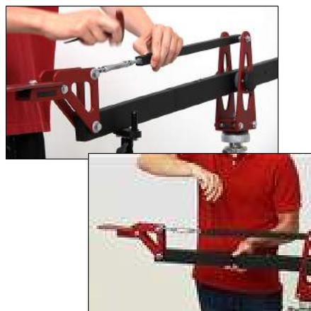
10. Connect the Turnbuckle on the Camera Platform beam to the female end of the Para Beam using the Hex tool and set screw.
